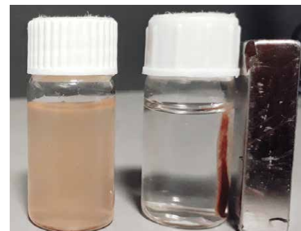
Solution of magnetic polymeric networks, used to remove the pollutants from water sources
